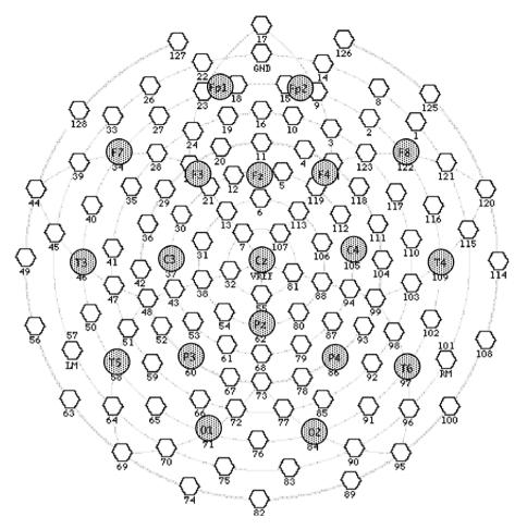
Fig. 1. Electrode locations. Standard 10-20 locations are marked in gray.
